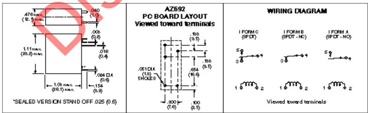
Dimensions in inches with metric equivalents in parentheses. Tolerance: ± .010"
